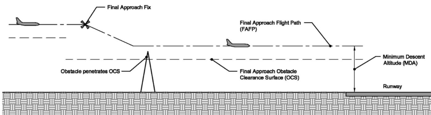
**Before Introduction of Step-Down Fix - Obstacle Penetration**
