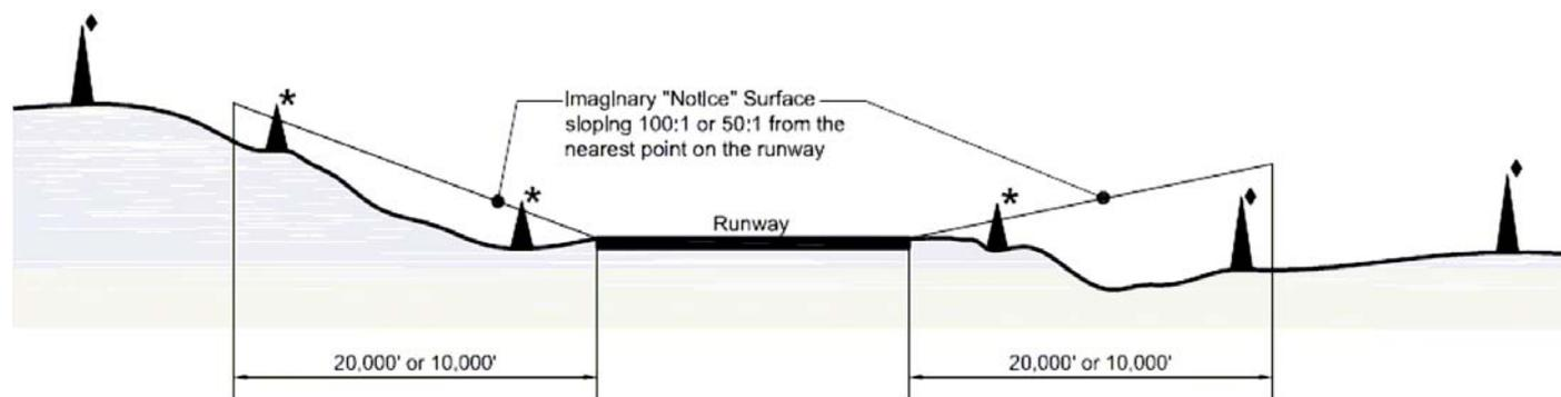
◆ §77.13(a)(1) Any proposed construction or alteration more than 200 feet in height above ground level (AGL) at its site requires notice
