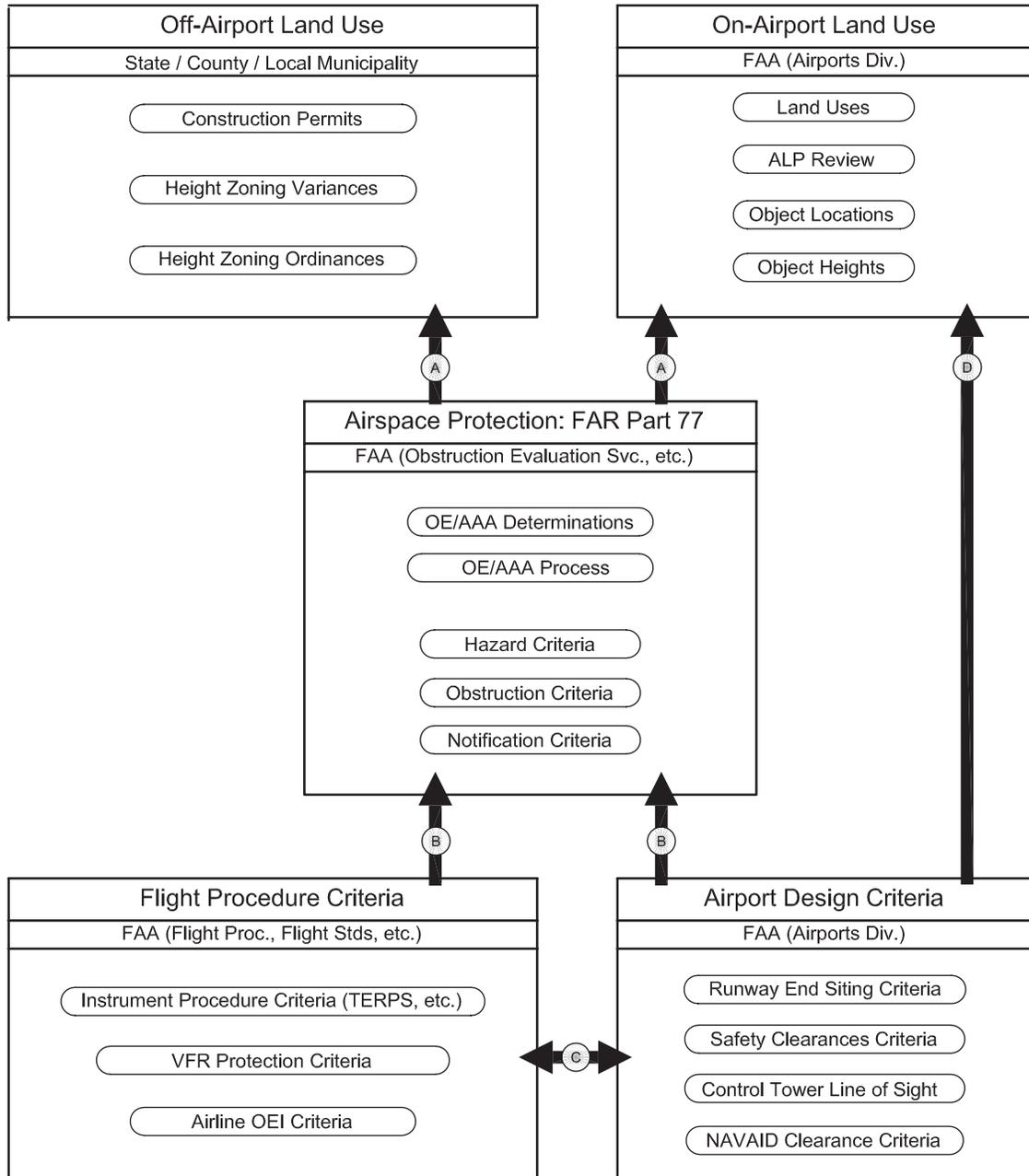
This diagram illustrates the interrelationships among various criteria and processes that function to protect airspace by limiting object heights. Arrows indicate a criteria or process influences another criteria or process; reading in the reverse direction of an arrow indicates "is based on"
