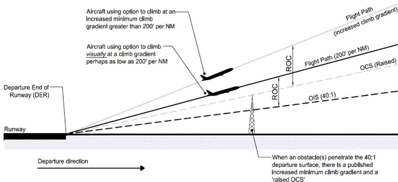
**Figure A.11.** Illustration of flight paths, obstacle identification surface (OIS), obstacle clearance surface (OCS) and required obstacle clearance (ROC) concepts, as applied to TERPS obstacle departure procedures.
