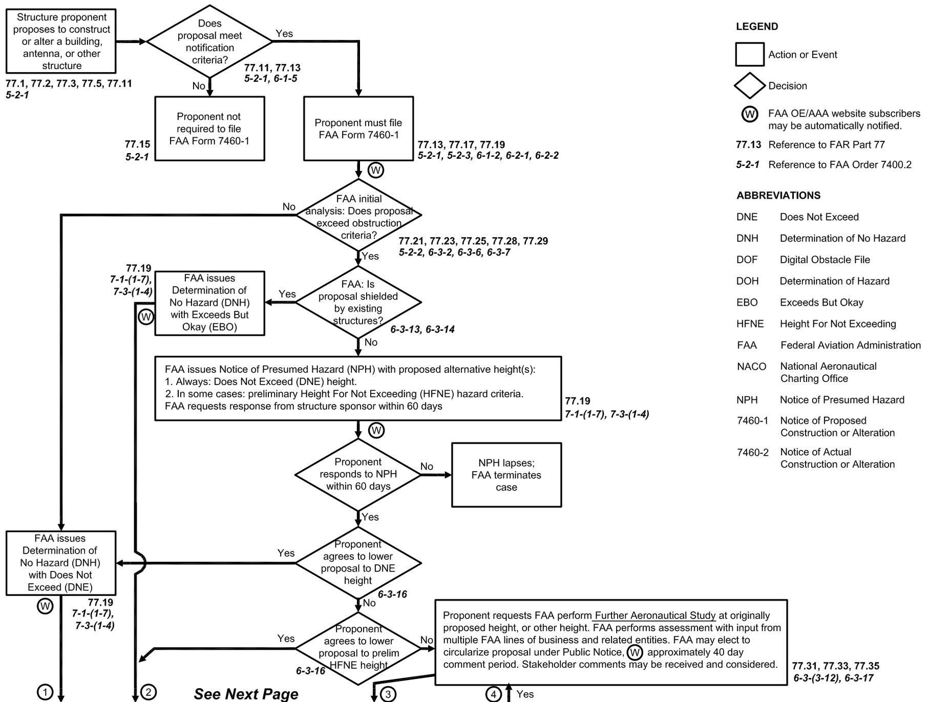
**Figure C.2. The FAA's obstruction evaluation/airport airspace analysis process.**
